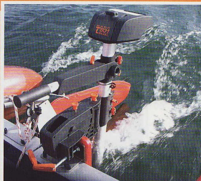
▲ The Torqeedo 801 short shaft electric outboard is unlike anything else: able to be dismantled, very light and efficient, it is a viable alternative to petrol outboards
